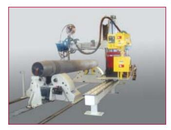
The system requirements included both step-over and spiral overlay and tapered surfaces at up to 2" per foot. Internal overlay requirements were for diameters as small as 15" and up to 12" in depth. The turning rolls utilized for the system are the exclusive Pandjiris Missouri Mule series with vertical adjustment to provide precision alignment of the propulsion shaft for the overlay process.
