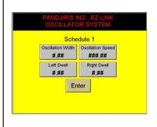
**Oscillator Schedule Setup:** There are 4 Schedule Setup Screens. The one displayed is "Oscillator Schedule 1". This screen allows the operator to set
