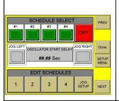
Oscillator Setup Screen: Allows the operator to setup all and edit 4 oscillator sequence programs. F1-F4 keys allow the operator to switch to a different Oscillation Sequence "on-the-fly". The "Oscillator Start Delay" parameter allows the operator to set a preset delay time from the arc start to the start of oscillation. Oscillator slide jog can be done with the joystick operator on the front of the control. If the "off" button is pressed, no oscillation will occur during the weld cycle.
