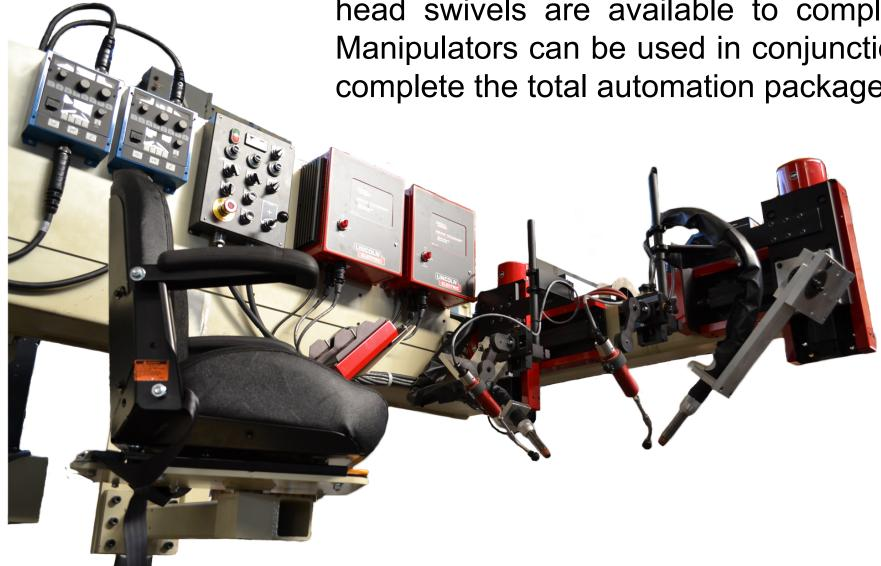
Pandjiris manipulators are an extremely versatile tool. Whether used with MIG, TIG, SAW, or Plasma, Pandjiris manipulators are a consistent and solid means of bringing the weld head to the work piece. Linear bearings are used on the Series 1100, 1400, 1600 and 2000 manipulators for improved stability and travel characteristics.
