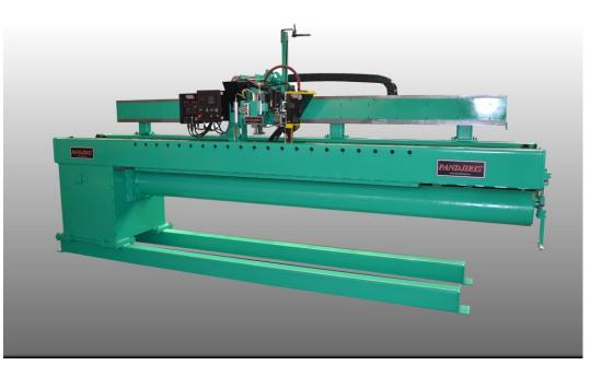
Pandjiris manufactures External, Internal and Flatsheet Seamers from 24" to 710" weld lengths utilizing most weld processes designed for making 100% penetration, single pass welds on cylinders and flat sheet minimizing or eliminating heat distortion to the material.
