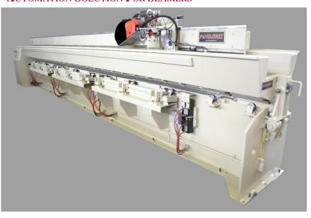
This Model 300-I/44-FS Internal/Flat Sheet Seamer is capable of welding Material 12 gage to 3/8" thick and up to 25' 0" in length. Both aluminum and stainless steel material with a minimum 44" inside diameter. The seamer can be equipped with the weld process of the customer's choice, including MIG, TIG. SAW and PAW.
