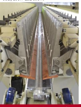
Pandjiris value added 4 Bar Linkage Clamping System for 44" minimum inside diameter shells provides 560 pounds per linear inch of clamping force at 80 PSI input pressure.
