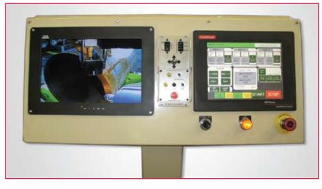
The new controllers are a PLC-based control designed to give the operator complete system control, flexibility, program storage, and simplicity at his finger tips.
